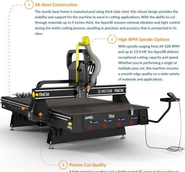
A high-precision gearbox and a tightly tuned AC servo motor system on 25mm linear rails with a helical rack. This configuration ensures very low backlash and delivers pristine cut quality with precise accuracy.
